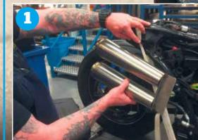
Starting with a pair of GFMoto S1000RR end cans, eoff Rayner works out where to put the collector – the part that takes converts the two pipes into one, then back into the two end cans.
