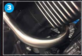
Reaching the front cylinder is straightforward, so Geoff bends the first primary so it runs under the air filter whilst also allowing access to the oil filler cap, and keeping in mind the need for ground clearance.
