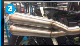
Geoff then expertly tig welds the collector unit then works out how much pipe he needs to reach the cylinders. As weight is not as much of a consideration he's working in T304 stainless steel.
